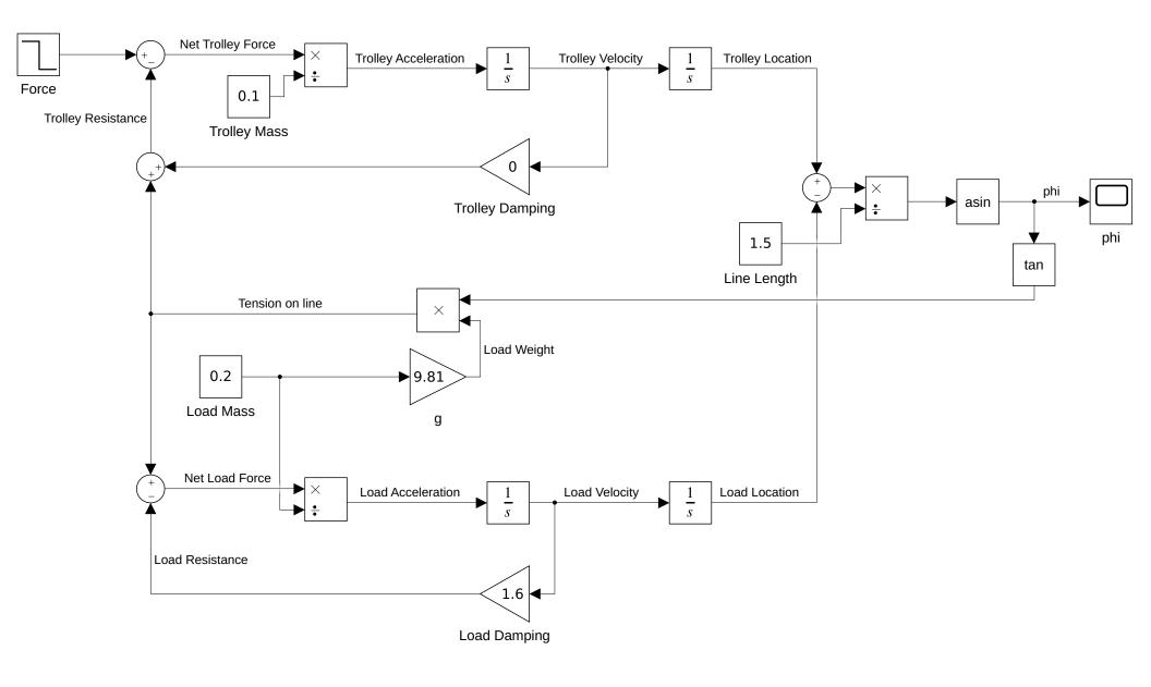
2.c) Transfer function linking \$\Phi\$ to \$\pi\_\tau\$. Linearize the system assuming \$\Phi \approx 0\$ prior to Laplace transform. When  $\phi \approx 0 : -\sin(\phi) \doteq \phi$  $\therefore$   $+an(\phi) = \phi$  $cos(\Phi) \doteq \# \{$ Linearized functions for the system:  $F = \ddot{x}_{T}m_{T} + \dot{x}_{T}b_{T} + m_{L}g\phi$   $m_{L}g\phi = \ddot{x}_{L}m_{L} + \dot{x}_{L}b_{L}$   $x_{L} = x_{T} - L\phi$ (1)(2) (3) $\begin{array}{lll}
